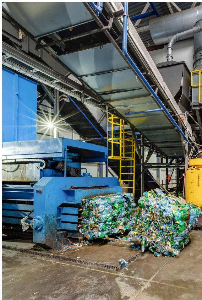
When fractions are being agglomerated by means of baling presses and briquetting systems, the materials that were separated from one another beforehand are bundled together for further treatment.
