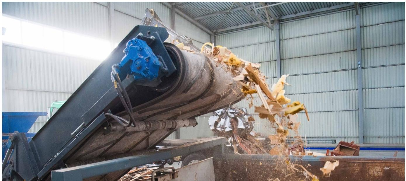
For the purposes of recycling the materials must be separated, sorted and sometimes prepared. In order to obtain the so-called separated fractions, a multitude of various stages are required. In doing so a wide variety of equipment and machinery is used, such as vibrators, drum sieves, magnets, shredders, grinders or air sifters.
